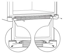
B Turn the leveling legs clockwise to raise the refrigerator, counterclockwise to lower it.
