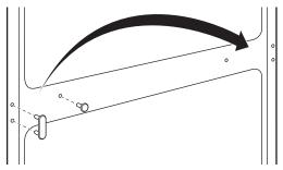
B A new hinge bracket is required for the left side (supplied in the door hinge kit). Install the center hinge from the kit on the left side.
