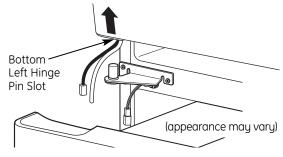
On left-hand doors, pass the wires and water line through the center hinge pin. Then connect the water line and 4-pin connector.
