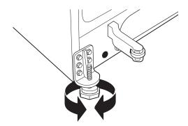
A CAUTION: To avoid possible personal injury or property damage, the leveling legs must be firmly touching the floor.
