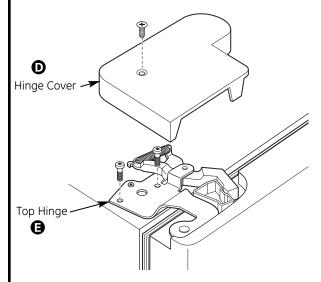
Remove the tape and tilt the door away from the cabinet. Lift the door off the center hinge pin. Ensure that the plastic hinge pin thimble remains on the hinge pin or inside door hinge pin hole located in the bottom of the door.
