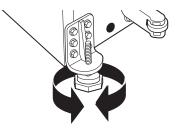
If the doors remain uneven, turn the adjustable pin to raise, or lower, the left door to match the right door. Use a 1/4" Allen wrench to turn the pin.
