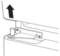
G Set the door on a non-scratching surface with the inside up.
