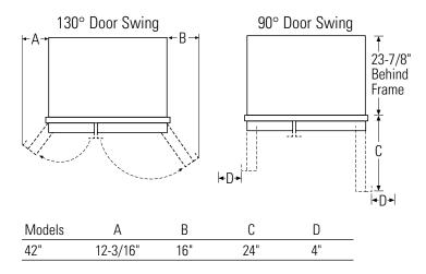
Allow minimum clearances for Freezer door (Dimension A) and Fresh Food door (Dimension B) for a full 130° door swing and to allow for drawer removal.
