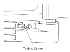
**IMPORTANT:** The vented toekick must remain unobstructed for proper air circulation.
