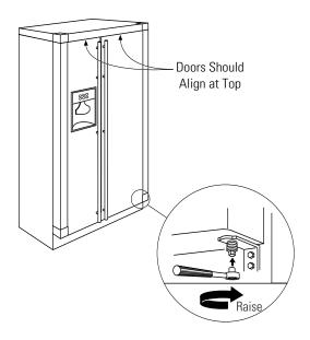
**NOTE:** A nylon plug is imbedded in the threads of the pin. The plug is designed to prevent the pin from turning. A wrench must be used to turn the pin.
