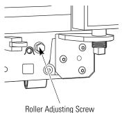
• Use a 3/8" hex socket or wrench to turn the adjustment screws. Turn the screws clockwise to raise the refrigerator, turn counterclockwise to lower it.
