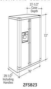
These Monogram free-standing refrigerators require the following clearances for proper air circulation, plumbing and electrical connections.
