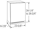
The product must be installed so that the custom panel front will project 2-3/4" forward of adjacent cabinets. This position will allow a full door swing and prevent interference with adjacent cabinetry. The opening between cabinets must be 23-3/4" minimum. These models can not be installed flush in 24"-deep cabinets.
