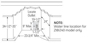
NOTE: If installing between frameless cabinets, a 1/2" wide filler strip or side panel may be needed on the hinge side. The filler strip will act as a spacer between the door case and adjacent cabinet and will prevent interference with the cabinet door swing. The width of the opening must include the filler panels.
