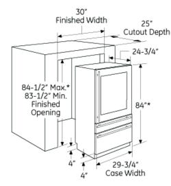
\* 84" high installation. The wine reserve can be adjusted to fit into a cutout that is 83-1/2" min. to 84-1/2" max. with the appropriate door kit. Use leveling legs and wheels for a maximum 1" height adjustment.
