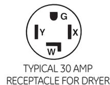
The power supply must be protected with 30 Amp fuses or breakers. It must be well grounded and conform to local codes.
