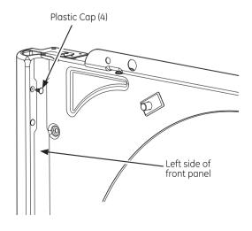
Remove the bottom screw from each hinge (right side) and partially insert them into the top left side hinge holes.
