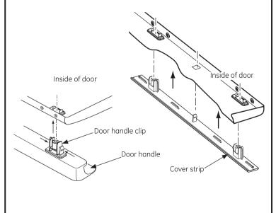
When the cover cap and door handle in place, mount the inner door back into the outer door with the screws removed in step 4. Make sure you mount the hinges on the side opposite the handle.
