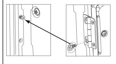
Loosen the bottom 2 right side hinge screws. Remove the door and place it on a protected flat surface to avoid any damage.
