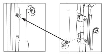
Loosen the bottom 2 right side hinge screws. Remove the door and place it on a protected, flat surface to avoid any damage. Remove both the Blind Plate and the Strike Plate and install them in opposite positions.
