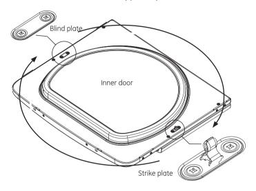
Remove the 4 door hinge screws, 8 edge screws, and 4 inside screws. Lift the inner door upwards using a flat blade screwdriver.
