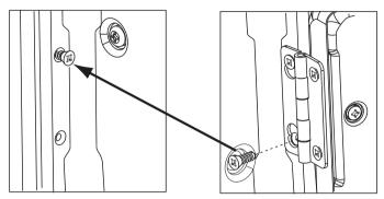
Loosen the bottom 2 right side hinge screws. Remove the door and place it on a protected flat surface to avoid any damage. Remove both the Blind Plate and the Strike Plate and install them in opposite positions.
