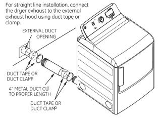
NOTE: WE STRONGLY RECOMMEND SOLID METAL EXHAUST DUCTING. HOWEVER, IF FLEXIBLE DUCTING IS USED IT MUST BE UL-LISTED METAL, NOT PLASTIC.
