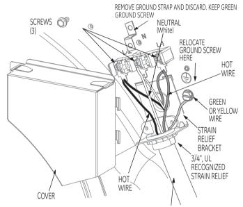
3 #10 AWG MINIMUM COPPER CONDUCTORS OR 120/240V 30A POWER SUPPLY CORD KIT MARKED FOR USE WITH DRYERS & PROVIDED WITH CLOSED LOOP OR SPADE TERMINALS WITH UPTURNED ENDS (NOT SUPPLIED).
