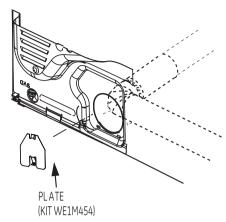
Connect standard metal elbows and ducts to complete the exhaust system. Cover back opening with a plate (Kit WE1M454) is available from your local service provider. Place with dryer in final location.
