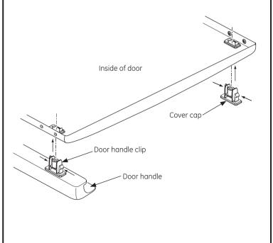
When the cover caps and door handle in place, mount the inner door back into the outer door with the screws removed in step 4. Make sure you mount the hinges on the side opposite the handle.
