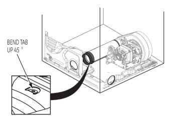
Through the rear opening, locate the tab in the middle of the appliance base. Lift the tab to about 45° using a flat blade screwdriver.
