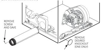
Detach and remove the bottom, right or left side knockout as desired. Remove the screw inside the dryer exhaust duct and save. Pull the duct out of the dryer.
