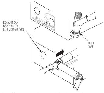
• Apply duct tape as shown on the joint between the dryer internal duct and the elbow.
