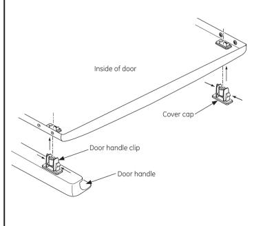
When the cover caps and door handle in place, mount the inner door back into the outer door with the screws removed in step 4. Make sure you mount the hinges on the side opposite the handle.
