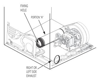
Reconnect the cut portion (A) of the duct to the blower housing. Make sure that the shortened duct is aligned with the tab in the base. Use the screw saved previously to secure the duct in place through the tab on the appliance base.
