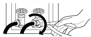
**9.** Check for leaks around the "Y" connector, faucet and hose couplings.
