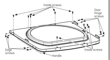
Mount the assembled door on the 2 upper left side hinge screws installed in step 2.
