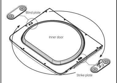
Remove the 4 door hinge screws, 4 edge screws, and 8 inside screws. Lift the inner door upwards using a flat blade screwdriver.
