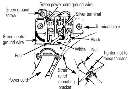
**⚠ WARNING:** Do not make a sharp bend or crimp wiring/conductor at the connections.
