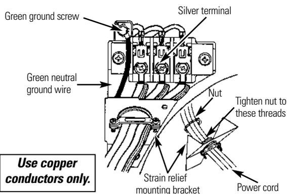
3. Thread a UL-listed 30A, 240V, 3 #10 AWG minimum copper conductor power cord through the strain relief.
