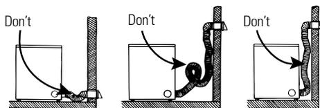
**WARNING** — The following are specific requirements for proper and safe operation of your dryer. Failure to follow these instructions can create excessive drying times and fire hazards.
