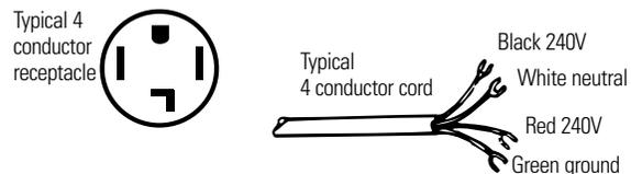
4. Thread a UL-listed 30A, 240V, 4 #10 AWG minimum copper conductor power cord through the strain relief.
