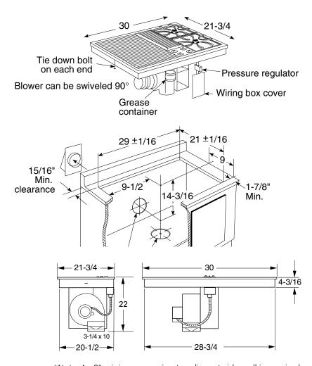
\*Note: An 8" minimum spacing to adjacent side wall is required
