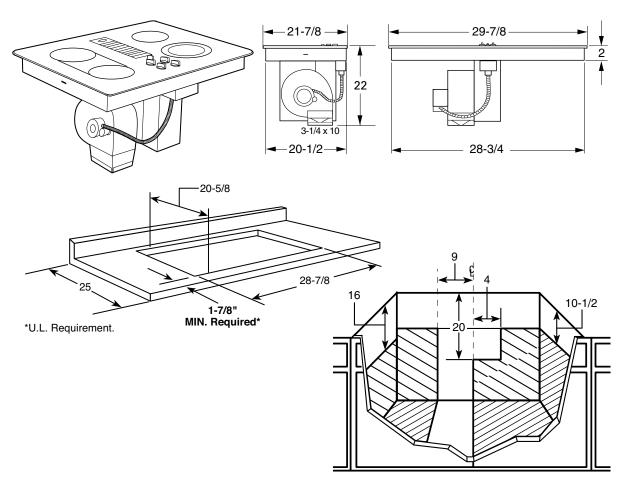
\*Note: A 6" minimum spacing to adjacent side wall is required Dimension and installation information are shown in inches.
