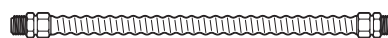
CSA-Approved Flexible Gas Line 3/8" Min. ID, 1/2" NPT Connection, 3-foot Maximum Length (Massachusetts Only)
