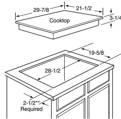
\*Depth of unit at conduit connection location (rear) is 6-1/2" on models PP980/950 and 4-5/8" on models PHP900/PP975/972/962/945/942/932/912, JP655/356/346.
