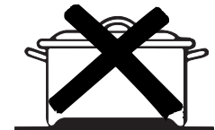
Pans with rounded, curved, ridged or warped bottoms are not recommended. Pan detection/sizing may not work properly with these types of pans.
