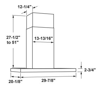
30" models require a 30"-wide opening \*The supplied duct cover fits 7'-7" to 10'-6" ceiling heights (12' ceiling height with optional high ceiling kit UX12DC93SS/UX12DC93TS) (14' ceiling height with optional high ceiling kit UX14DC93SS/UX14DC93TS)
