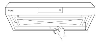
7. Reattach the metal grease tray to the range hood.
