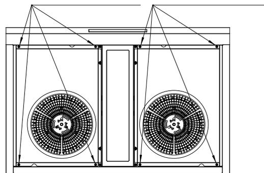
5. 6" Round Ducting: Remove the top cover (fig.1) and then fix the 6" round ducting (fig.2).
