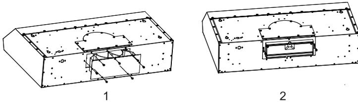
8. Measure the size of the outlet adapter relative to the cabinet and create an opening in the cabinet to let pass the outlet adapter and power cable. Make sure there is excess opening to accommodate electrical wires and hood exhaust. If you are installing the hood under the cabinet with a recessed bottom, it is advised to use a 4" wood fillers on both the sides.
