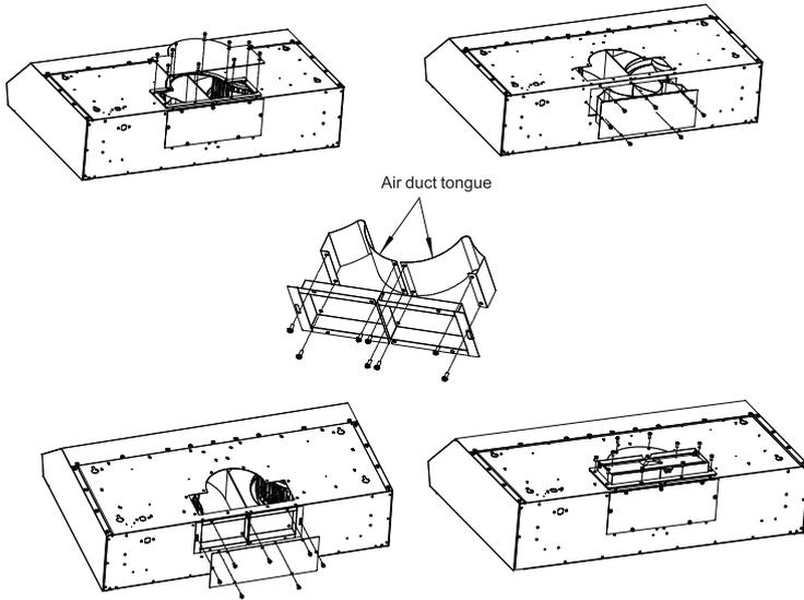
7. 10" x 3 1/4" horizontal ducting: Remove the back cover (fig.1) and then fix the ducting (fig.2).
