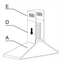
Chimney Top: Ensure the chimney mounting bracket (C) is securely attached to the wall. Raise the chimney top (E) up inside the chimney bottom(D). Secure the chimney top (E) to the chimney mounting bracket (C) with chimney mounting bracket screws (CC) from two sides.
