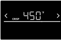
The Crisp mode can be activated and deactivated with a long press on **Crisp Mode**. In the crisping process, it's possible to start, when the set temperature of the oven is reached. The maximum duration of Crisp mode operation is 5 minutes.
