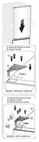
16. Connect electrical connector ① as shown in the picture, then fix part ② by screw ③ refer to step 2.
