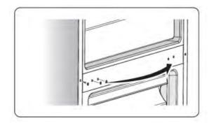
9.Lie the refrigerator backwards, Remove part ④ (right), Remove 3 self-tapping screws from the lower hinge -right.Unscrew the lower hinge-right axis then
