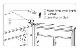
3. Remove the upper door from the middle hinge by carefully lifting the door straight up. Then place the upper door on a smooth surface with its panel upwards.
