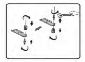
11. Stand the refrigerator upright and carefully slot the lower door onto the lower hinge-left pin and hold it in position. Install middle hinge-left (provided in the plastic accessory bag) and ensure the lower door in place.
