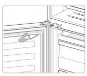
12. Carefully slot the upper door onto the middle hinge pin and hold in position. Move the upper door to an appropriate position, adjust the upper hinge-left (provided in the plastic accessory bag) and upper door, then fit the hinge pin into the hinge hole at the top of the upper door to secure it in place. Then fix the upper hinge part with screws (Please carefully hold the upper door by hand when installing)
