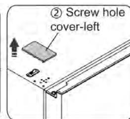
8. Change screw hole covers and screw on middle cover plate from left to right (as shown in figure below).
