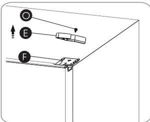
3. Remove the upper hinge (Please hold upper door by hand when installing).
