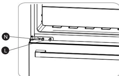
9. Screw out the upper hinge axis turn the upper hinge over and fix axis on it. Then place it at side for use.
