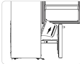
4. Remove the 2 screws attached to the supporting frame.
