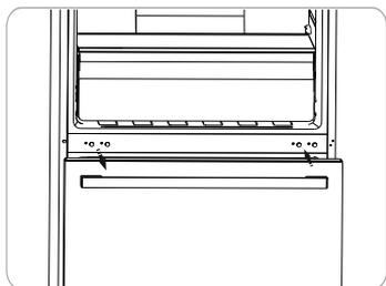
8. Put out the left middle hinge (N) (provided in plastic). Then screw it with 2 screws (L) from right side.
