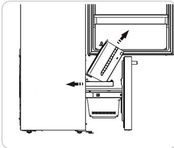
3. Remove the lower freezer drawer by lifting it up.
