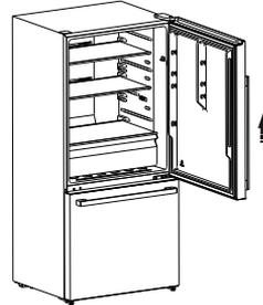
5. Loosen the two screws (G) on the right bottom of the fridge door, then take out the right stopper block (H) and the right door stopper (I). Then install the left stopper block (K) and the left door stopper (J) (provided in the plastic bag)
