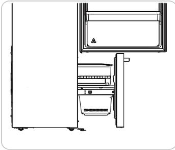
2. Take out the upper freezer drawer by lifting it up from the rail system, then push the rail system back.
