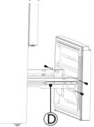
5. Pull out the freezer door and lift it up in the direction of the arrow.
