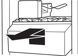
4. Replace the bin by pushing it in all the way or the dispenser will not work. Push the wire shutoff arm down to the ON position to restart ice production. Make sure the door is closed tightly.
