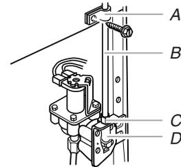
6. The ice maker is equipped with a built-in water strainer. If your water conditions require a second water strainer, install it in the ¼" (6.35 mm) water line at either tube connection. Obtain a water strainer from your nearest appliance dealer.
