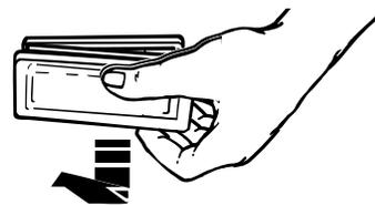
3. Remove bulb from socket by pulling straight out of the ceramic base.
