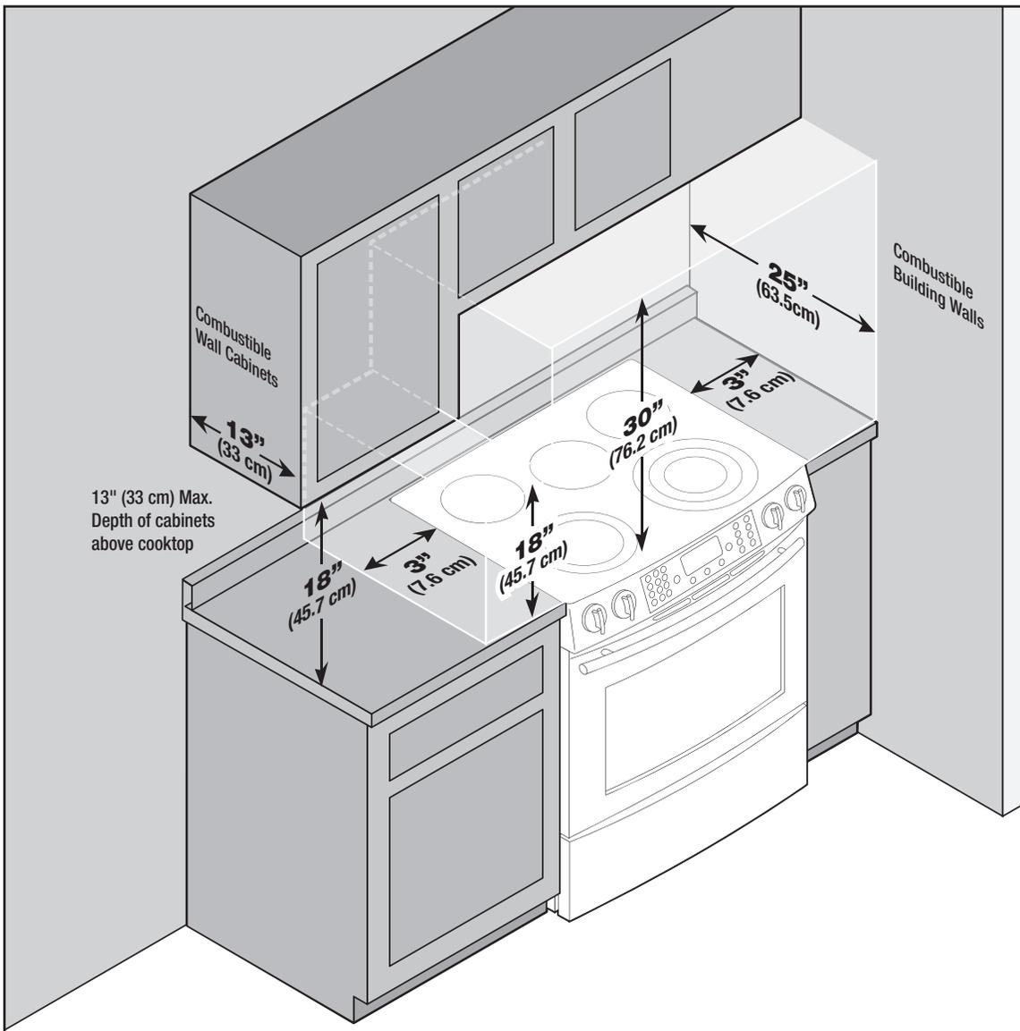
Range may be installed with 0" (0 cm) clearance adjacent to (against) combustible construction at the rear and on the sides below the cooktop.
