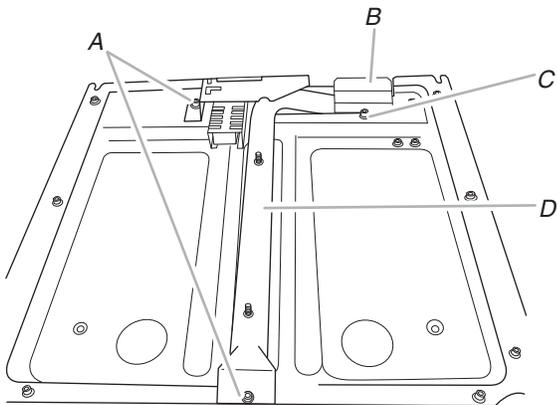
A. Oven bake burner screws      C. Orifice hood cover screw
