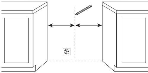
2. Check for obstructions before marking the vent hole location. Mark a horizontal line  $8\frac{3}{16}$ " (20.8 cm) from the floor. Mark a vertical line up to a maximum of  $2\frac{1}{4}$ " (7.9 cm) from the right side of the cabinet centerline.
