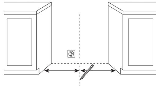
2. Position template on floor by matching the centerline of the template to the centerline drawn on the floor and place template  $2\frac{1}{4}$ " (5.7 cm) from the back wall.
