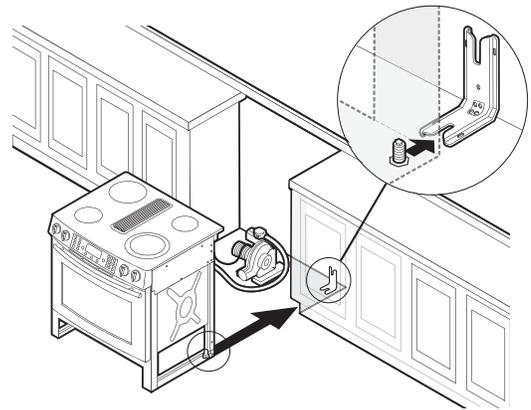
7. Check that the flexible connector and electrical cord are not kinked. Use a flashlight to look underneath the bottom of the range.
