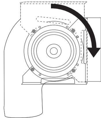
9. Position blower motor in cabinet opening and mount blower motor to the floor.
