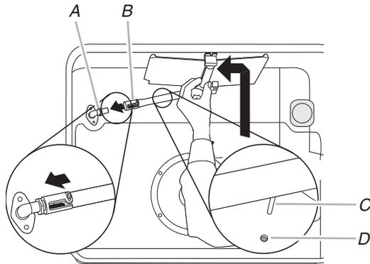
A. Oven broil burner orifice hood
