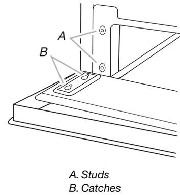
12. Insert downdraft vent filter and place vent grate over opening. Replace grates and burner caps.
