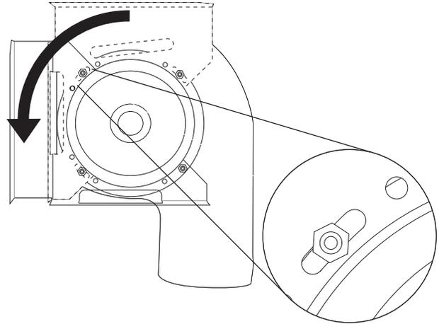
8. Remove the bracket from the other side of the blower motor, rotate 90° and secure with 4 locknuts.
