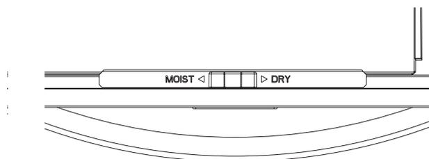
The Moist-Dry slide control allows you to open or close the vent slots in the door. The MOIST setting holds moisture in, while the DRY setting allows steam and moisture to escape from the drawer.
