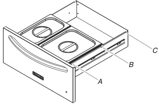
A. Position 1 pan support rail locator notch
