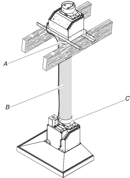
A. Vent transition - in-line smart kit (bottom)
