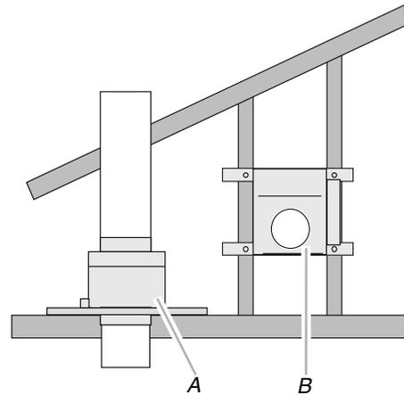
A. Mounted on top of ceiling joists (vertical duct)
