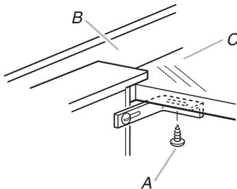
A. When attaching undercounter bracket to underside of countertop, make sure that the screw length will not go through countertop when tightened.
