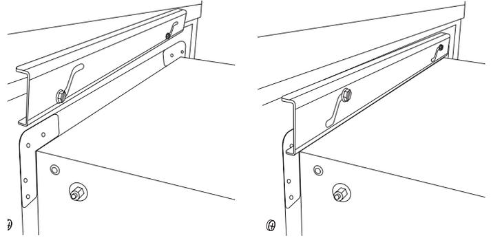
9. Reinstall panel to front side of vent box panel. Place bottom tab of the panel into the bottom mounting channel.
