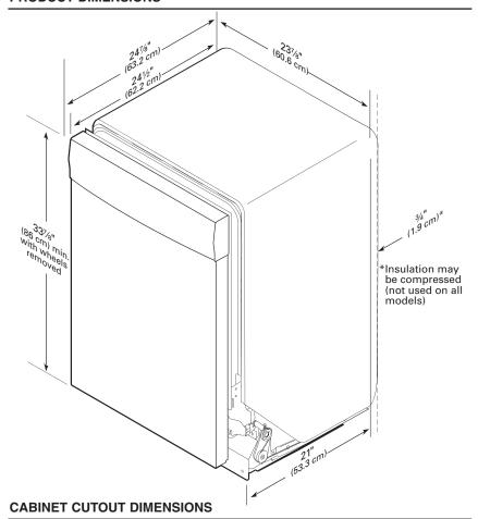
Corner locations require a 2" (5.1 cm) minimum clearance between the side of the dishwasher door and the wall or cabinet.
