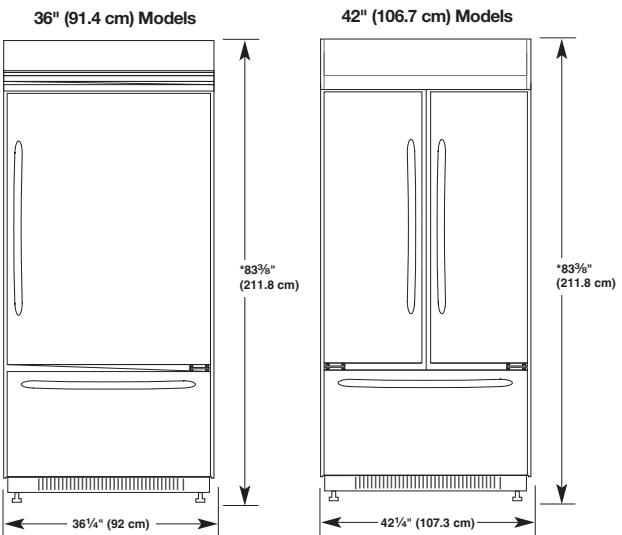
\* When leveling legs are fully extended to 1-1/4" (3.2 cm) below rollers, add 1-1/8" (2.9 cm) to the height dimensions.
