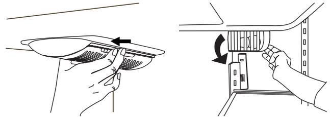
3. Replace burned-out bulb(s) with appliance light bulb(s) no greater than 40 watts.
