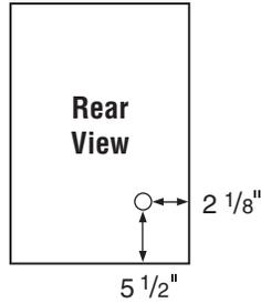
1/4" inlet water line. If water line is connected directly behind the icemaker, allow an additional 2" clearance
