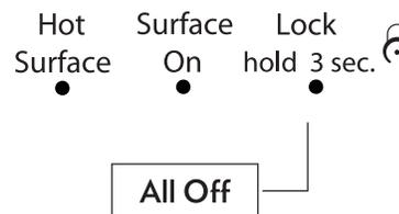
If the cooktop is on when a power failure occurs, the Hot Surface Indicator Light will remain on up to 45 minutes after the power is restored to the cooktop.
