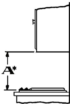
A = 24" (61 cm) minimum when bottom of wood or metal cabinet is protected by not less than 1/4" (0.6 cm). FLAME RETARDANT millboard covered with not less than no. 28 MSG sheet steel, 0.015" (0.4 mm) stainless steel, 0.024" (0.6 mm) aluminum or copper.
