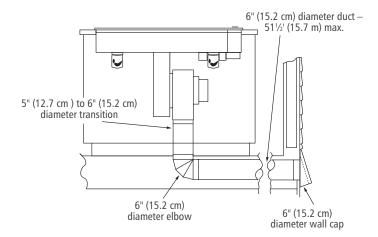
THROUGH FLOOR BETWEEN JOISTS TO OUTSIDE
