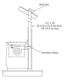
**REAR DUCTING IN WALL TO ROOF**
