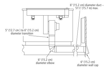
THROUGH FLOOR BETWEEN JOISTS TO OUTSIDE
