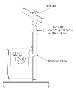
**REAR DUCTING IN WALL TO ROOF**
