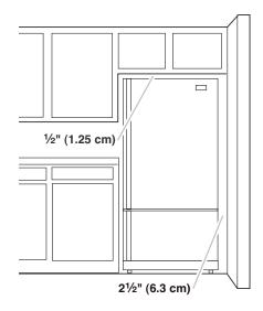
To ensure proper ventilation for your refrigerator, allow for 1/2" (1.25 cm) space on each side, at the top and behind the refrigerator. When installing your refrigerator next to a fixed wall, leave 2-1/2" (6.3 cm) minimum on each side (depending on your model) to allow for the door to swing open. If your refrigerator has an ice maker, allow extra space at the back for the water line connections.
