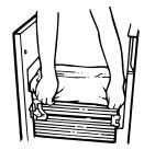
Lock bag in place by pulling the four prepunched holes over the bag retainer buttons. Holes will expand over the buttons without damaging the bag. 3. Press inside of bag against the drawer bottom, sides and corners for a smooth fit.
