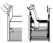
4. Place the other 2 corner posts on the floor to the side of the compactor. Grasp the sides of the compactor cabinet and put compactor on its side on top of the corner posts. Remove the shipping base from the bottom of the compactor.
