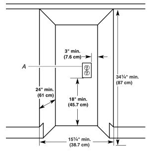
A. Grounded eletrical outlet must be a minimum of 3" (7.6 cm) away from surrounding cabinets or nearby walls as shown. It can be placed either to the left or the right side of the compactor.
