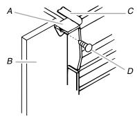
A. Mounting clip B. Cabinet C. Retaining bracket D. Mounting screw
