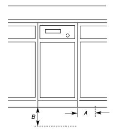
A. Leave 6" (15.2 cm) of clearance space to the right side of the compactor in order to remove the compactor bags.
