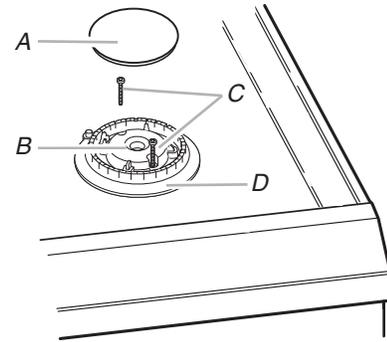
A. Burner cap      C. Burner base screws
