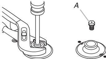
Use the following chart for correct LP gas orifice spud for each burner. Refer to the model/serial/rating plate behind the control panel for proper sizing of LP gas orifice spuds for each burner location.
