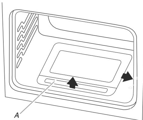
4. Lift up and remove oven bake burner cover.
