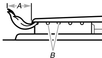
**Burner Ports:** Check burner flames occasionally for proper size and shape as shown in the previous illustration. A good flame is blue in color, not yellow. Keep this area free of soil and do not allow spills, food, cleaning agents, or any other material to enter the burner ports.
