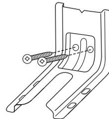
5. Using a Phillips screwdriver, mount the anti-tip bracket to the wall or floor with two #12 x  $1\frac{5}{8}$ " screws provided.
