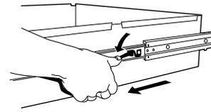
4. Holding the drawer by its sides, not its front, gently pull it all the way out.
