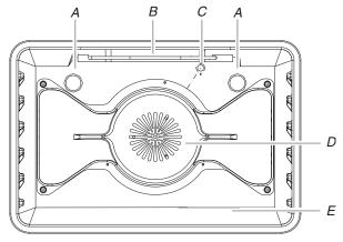
A. Oven lights B. Full and center broil elements C. Oven cavity sensor D. T.H.E.™ convection fan and element (on 807 and 907 models) E. CleanBake™ element (not visible)
