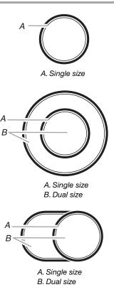
The Dual-Size Elements offer flexibility depending on the size of the cookware. Single size can be used in the same way as a regular element. The dual size combines both the single and outer element and is recommended for larger size cookware.
