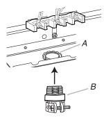
A. Removable retaining nut B. Conduit
