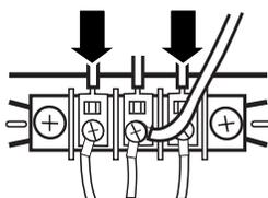
5. Tighten strain relief screws.
