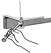
4. If the dryer is not level, move the dryer slightly away from the wall and first prop the front with a wood block and adjust the feet as necessary; then prop the back and adjust feet as necessary. Repeat this step until dryer is level.
