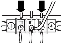
5. Tighten strain relief screw.
