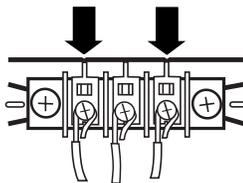
4. Tighten strain relief screw.
