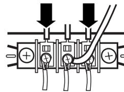
4. Tighten strain relief screws.
