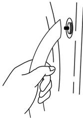
4. Push the handle against the door. Using a Phillips screwdriver, tighten the screws.
