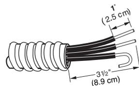
When connecting to the terminal block, place the hooked end of the wire under the screw of the terminal block (hook facing right), squeeze hooked end together and tighten screw, as shown.
