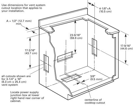
Vent system cutout dimensions for internal blower models only. Exterior mounted blower systems connect with 10" (25.4 cm) round vent. The cutout locations for this vent system will depend upon your specific installation.
