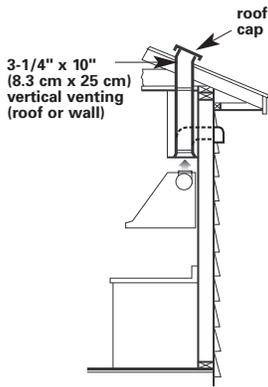
The vent system length should not exceed the lengths shown in the chart below.
