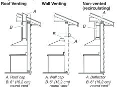
\*The 48" (121.9 cm) hood uses two 6" (15.2 cm) round vents or transitions to 10" (25.4 cm) round vent using Part Number 4396915.
